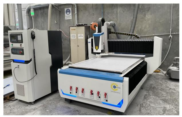
MC series CNC router is Fully featured CNC routing machine with 3D capability designed for small to medium size work in a variety of materials. It offers advanced features and flexibility suited to manufacturers in many different industries.
